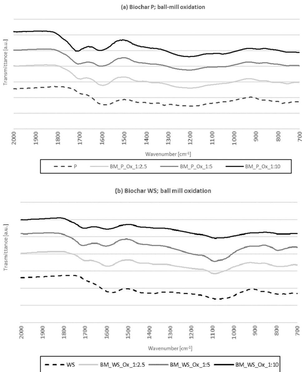
Fig. 1 FTIR spectra of P (a) and WS (b) biochars, oxidized with the ball mill method at different Oxone® concentration
