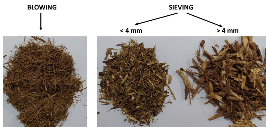
Figure 1. Biomass fractions obtained after the separation process.
