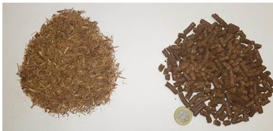
Figure 3. Appearance of J. communis material before and after the pelletisation process.
