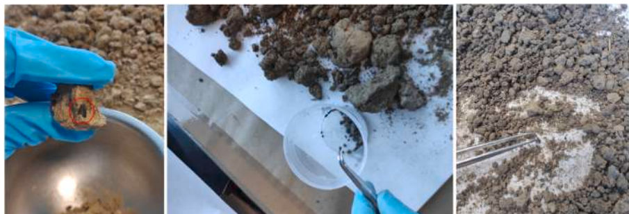
Fig. 8. Biochar manual recovery from soil samples.
