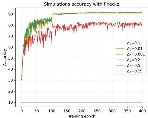
Fig. 2. Accuracy for different \Delta_0 values in the fixed- \Delta scenario. Initial \Delta values above 0.1 yield sub-optimal accuracy.
