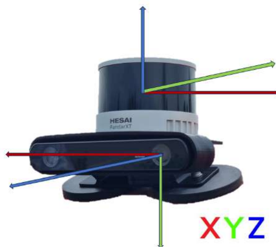
Figure 3. Hesai PandarXT-32 LiDAR and Stereolabs ZED2 camera integrated sensors' setup.
