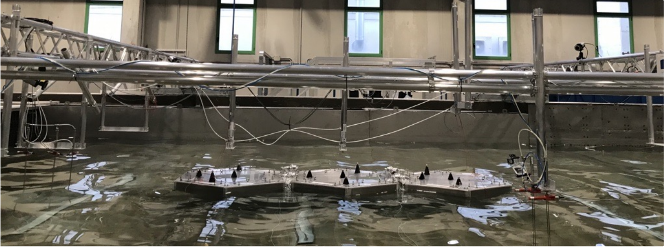
Figure 8: The MMFS tested system during an operative sea state experiment at the LIDR facility.
