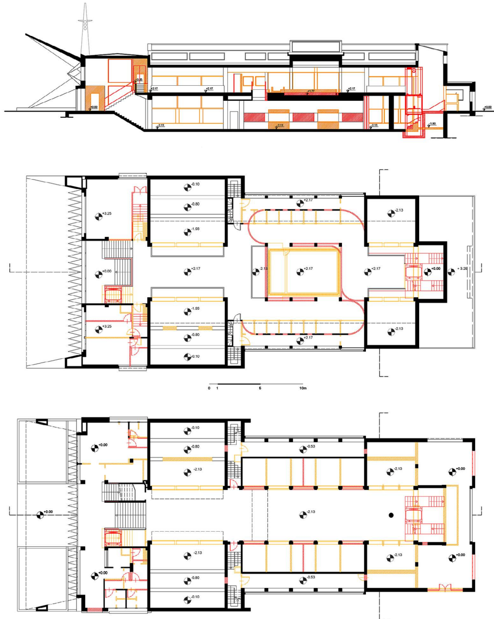
Fig. 5 - Demolition and construction for the Museum of Japanese Comics and Animation design project inside Enzo Venturelli's aquarium-retailarium. From the bottom ground floor, first floor, and longitudinal section view (Author: V. Bottari).
