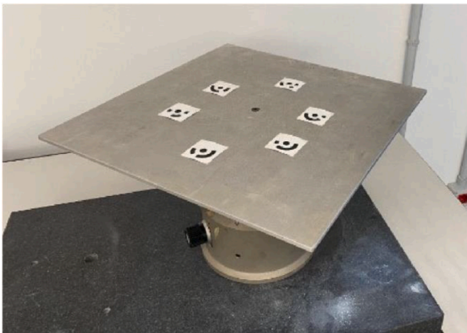
Fig. 3. Rotary table employed for the photogrammetric process located within the Manufacturing Industry 4.0 Laboratory (MInd4Lab) at the Politecnico di Torino.
