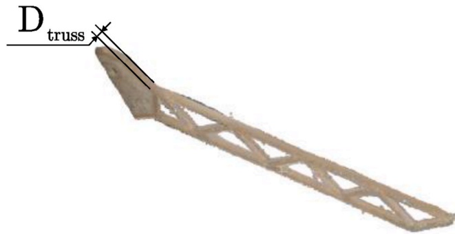
Fig. 7. Reconstructed point cloud of the truss with the definition of D_{truss} .
