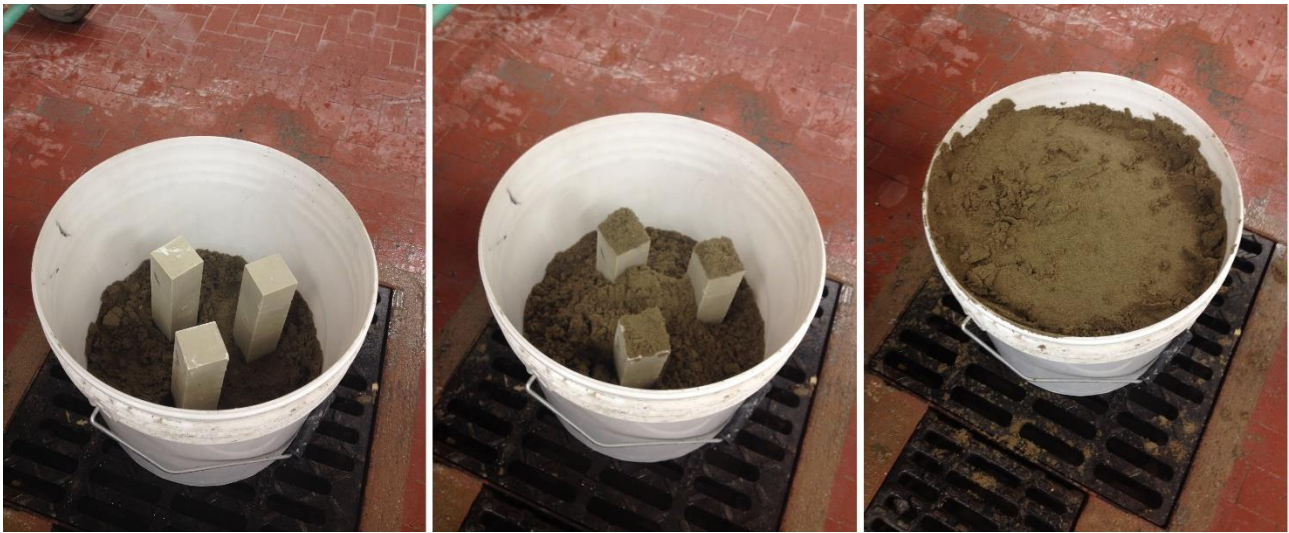
Figure 2. Burial process for samples of two-component grout under modalities 2 and 3.
