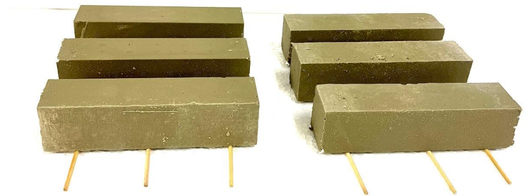
Figure 4. Samples cured under the action of air. The small wooden cylinders allowed air to reach the bottom of the samples. These samples were produced for mechanical assessment.
