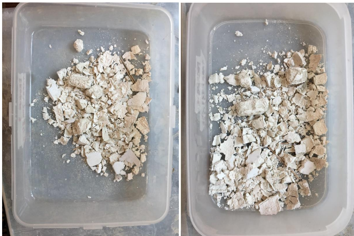
Figure 13. Tested samples of two-component grout after about two months of curing.
