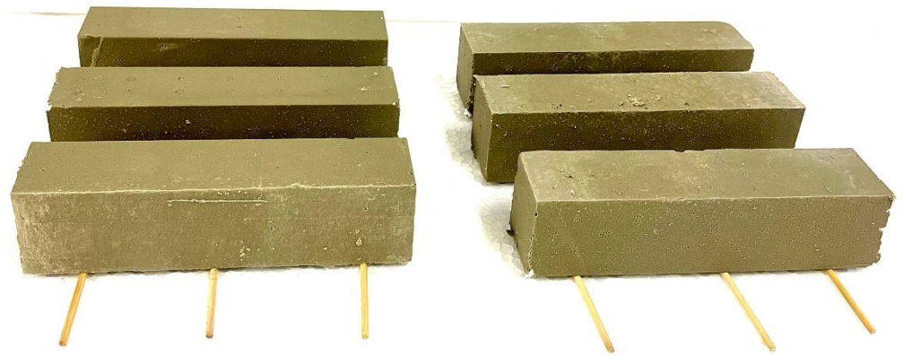
Figure 4. Samples cured under the action of air. The small wooden cylinders allowed air to reach the bottom of the samples. These samples were produced for mechanical assessment.
