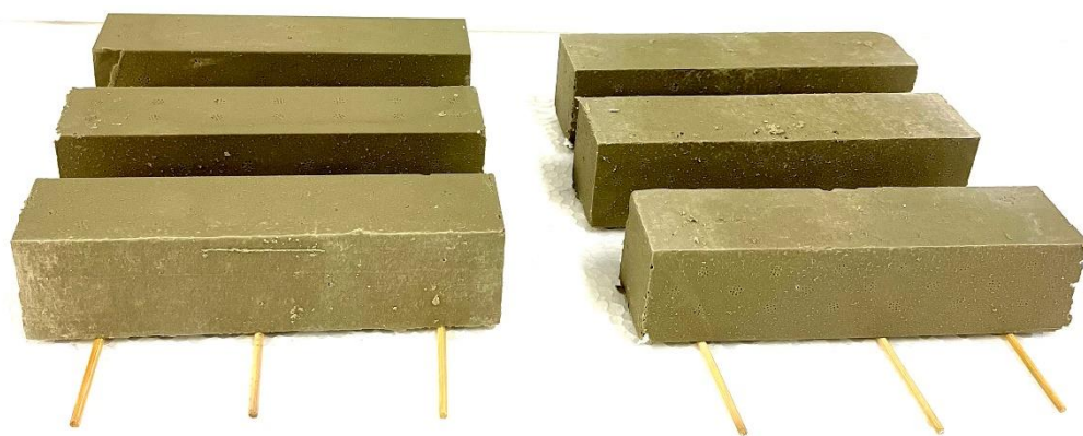
Figure 4. Samples cured under the action of air. The small wooden cylinders allowed air to reach the bottom of the samples. These samples were produced for mechanical assessment.
