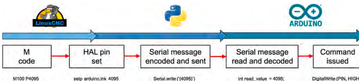
Fig. 6. Summary of the pipeline to send a command from LinuxCNC to an Arduino board connected to the PC through serial communication showing an example of user defined M command to control the inkjet toolhead in the BOOST bioprinter (i.e., M100 P4095).
