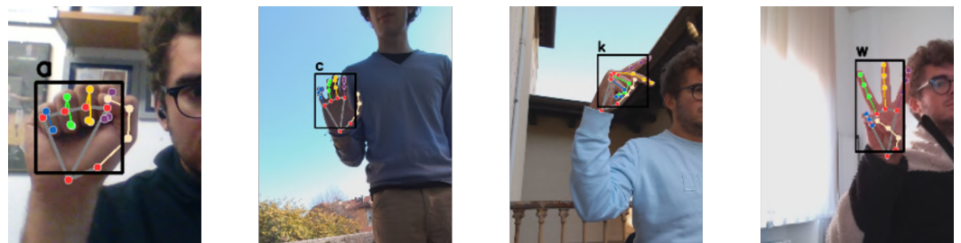
Figure 10. Qualitative tests in real-world uncontrolled settings. Different colors refer to different subgroups of hand landmarks.
