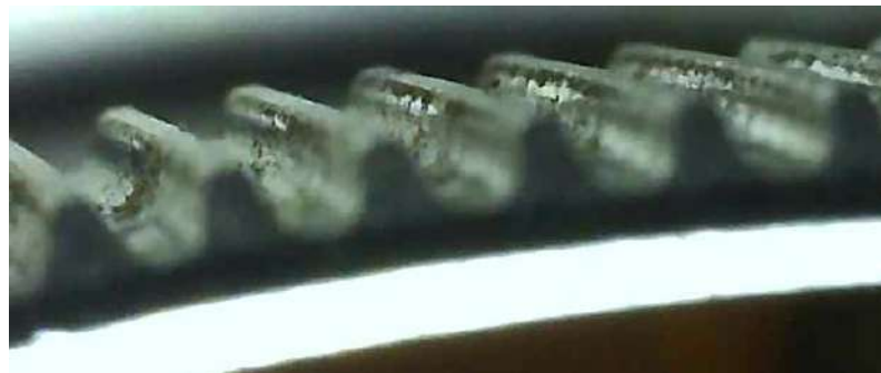
Figure 5. Pitting of the flexspline teeth detected on the shoulder joint of a UR5 collaborative robot.
