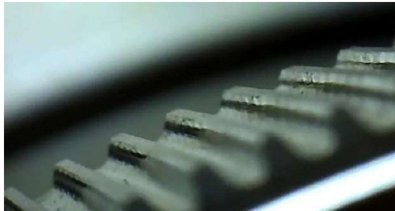
Figure 10. Flexspline tooth cracks.
