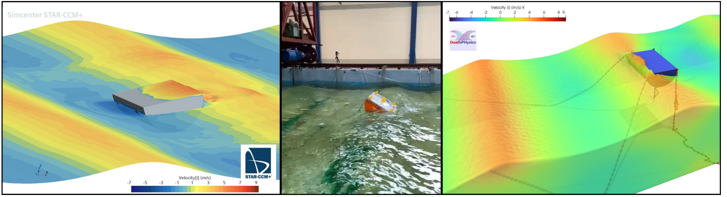
Figure 6: On the left the model developed with STAR CCM+ (the mooring is not visible but it is present in the model). In the middle the experimental campaign performed in 2021. On the Right the model developed with DualSPHysics
