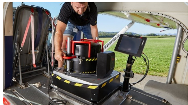
Figure 3: Data acquisition for Turin DT project with Leica CityMapper-2
