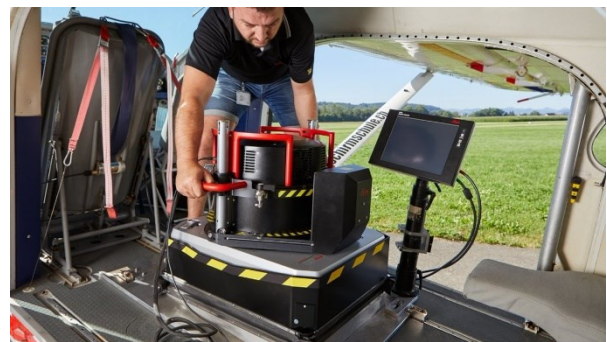
Figure 3: Data acquisition for Turin DT project with Leica CityMapper-2
