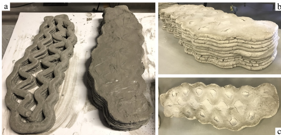
Fig. 1. Fresh-state components (a): 3D printed path and multi-density component; hardened-state multi-density component (b, c).
