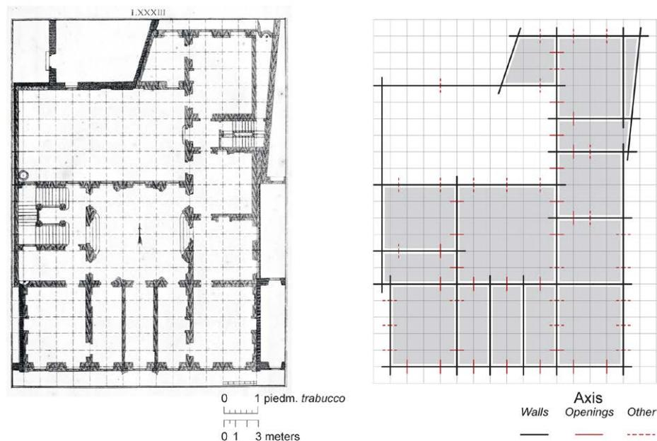
Fig. 6. Application example for «stabilire le parti degli Edificj» using the squareness method (Vittone 1760, Plate LXXXIII). Elaboration by the author.
