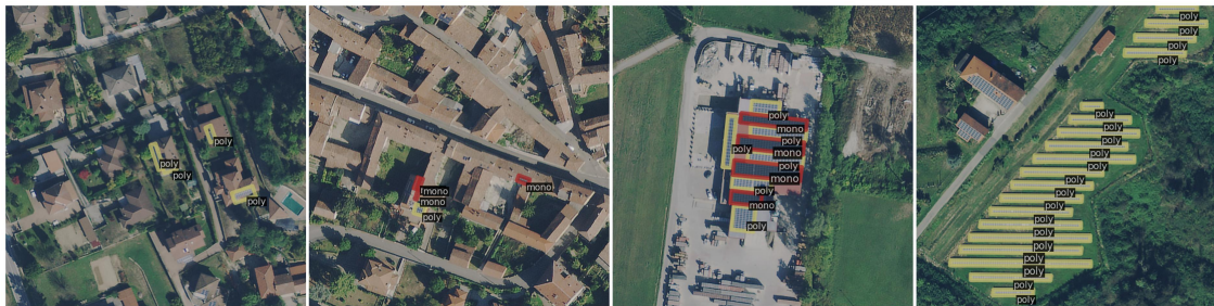
Figure 4.5: Examples tiles extracted from the dataset, together with their annotations. Starting from the left, the first two images show the smaller domestic installations, while the last two illustrate larger industrial plants.
