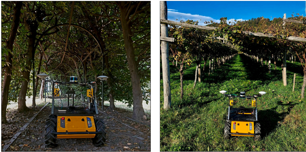
Fig. 1. The proposed SegMin and SegMinD algorithms allow to precisely guide an autonomous mobile robot through a dense tree row solely using an RGB-D camera. An arched hedge is shown on the left, and a pergola vineyard row on the right.
