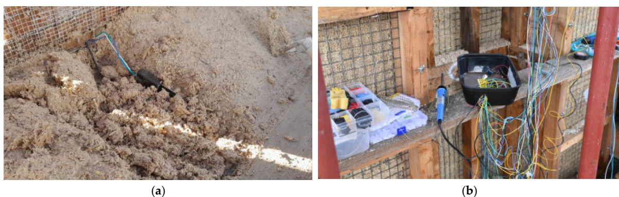
Figure 6. Pictures showing the work of placing the probes: (a) embedding the probes and (b) welding the hardware system.
