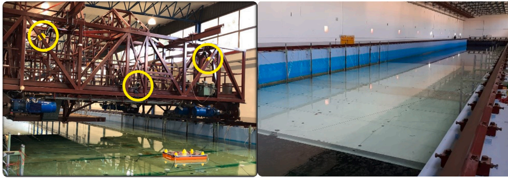
Fig. 4. On the left, the dynamometric carriage from which the acquisitions are made, with PeWEC in the water. The yellow circles indicate the cameras of the Qualisys system. On the right, an image of the artificial seabed.
