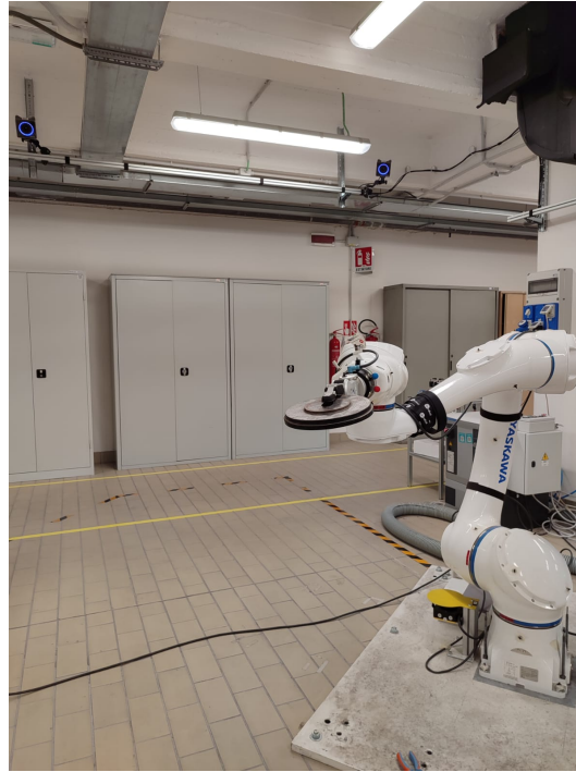
Figure 7. Yaskawa cobot and OptiTrack cameras (black cubes with a blue ring in the picture) used for the DT case study.
