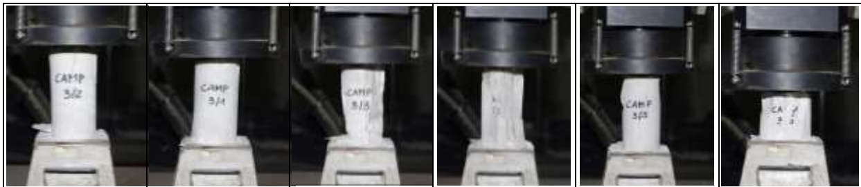
Figure 1. Samples under the UCS test.
