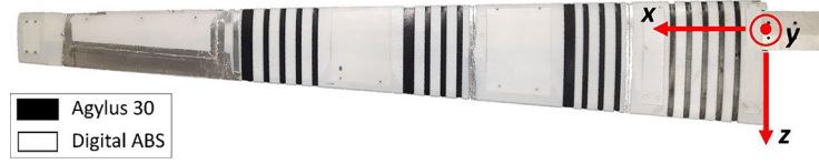
Figure 4 XB-2 wing top view. y-axis coming out of the page
