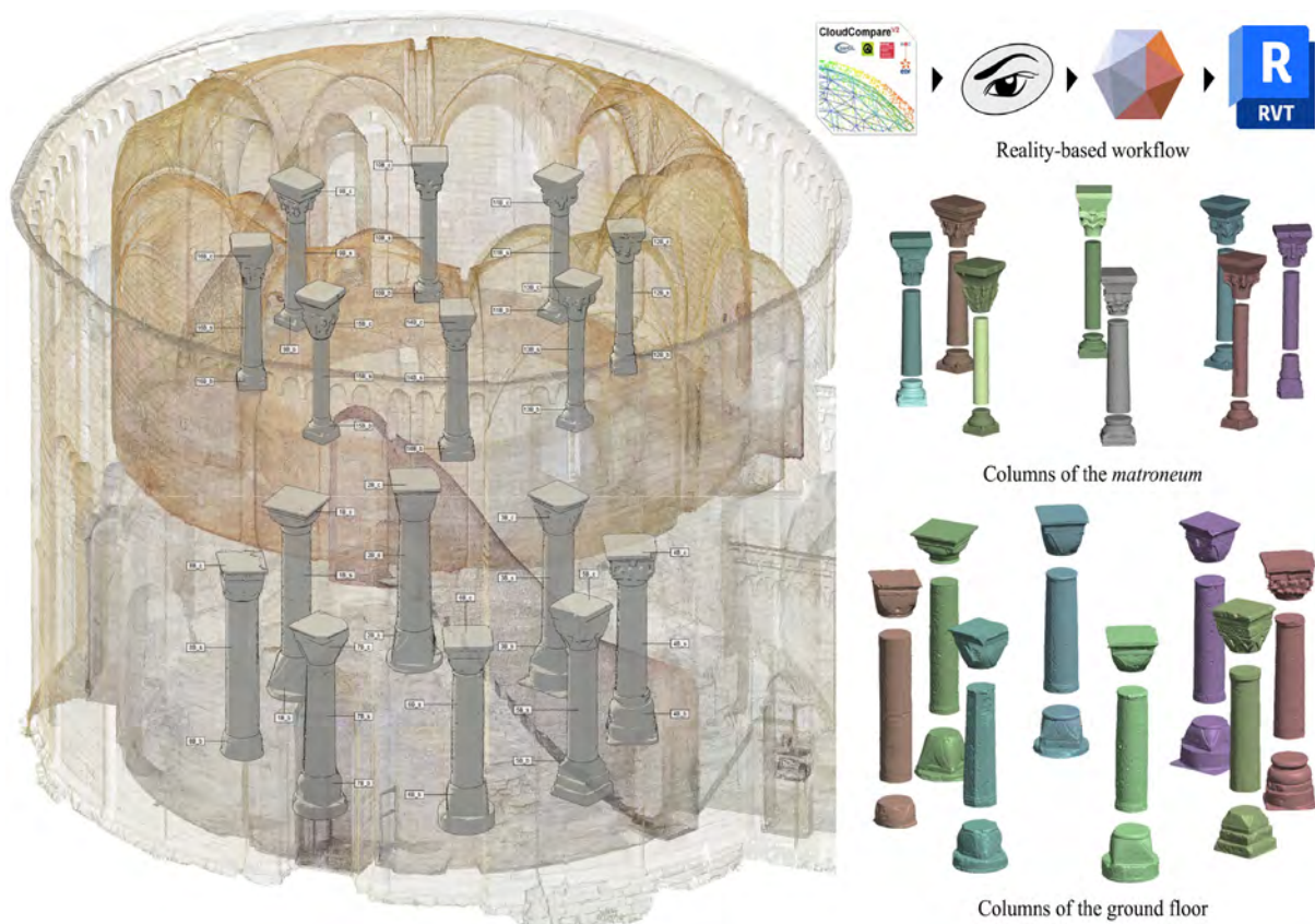
Fig. 5 - Semantic segmentation of the column elements encoded according to Rota Nodari [27]. From the left, superimposition between HBIM models and points cloud. On the right, reality-based segmented models. (@E.C. Giovannini).
