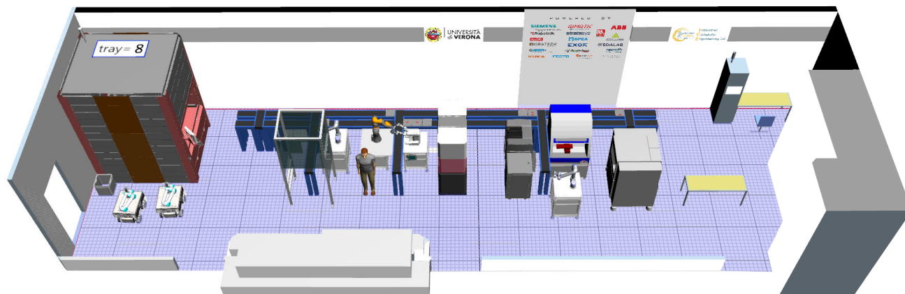
FIGURE 5. The ICE laboratory visualized in the Digital Twin tool. The 3D environment has accurate 3D models of all the devices and machinery existing in the real world with the same sizes.
