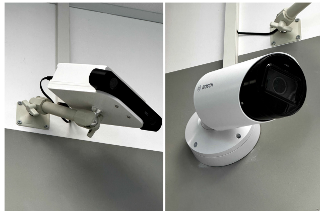
FIGURE 4. The cameras mounted in the laboratory. On the left: the Zed RGB-D camera with the Jetson board in its enclosure. On the right: the RGB Bosch camera.
