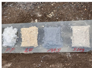
Fig. 2. Polypropylene fiber (P.P), Zeolite (ZE), Micro Silica (MS) and SLAG used in FRSCC mixes.
