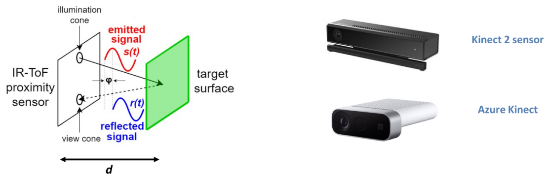
Figure 2. ToF Sensor Mechanism and Kinect Devices. Left: IR-ToF sensor mechanism with emitted and reflected signals. Right: Kinect 2 and Azure Kinect devices using ToF technology for depth sensing.
