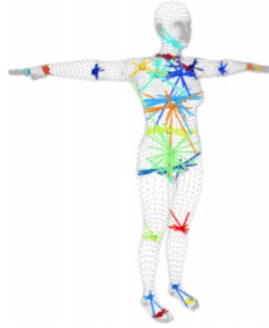
Figure 26. Estimation of joint centers positions. The left knee joint is computed as the weighted average of red vertices.
