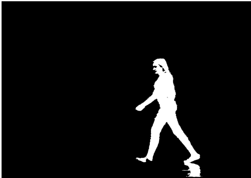
Figure 14. Segmentation mask obtained after the small areas' removal. The largest area is the subject.
