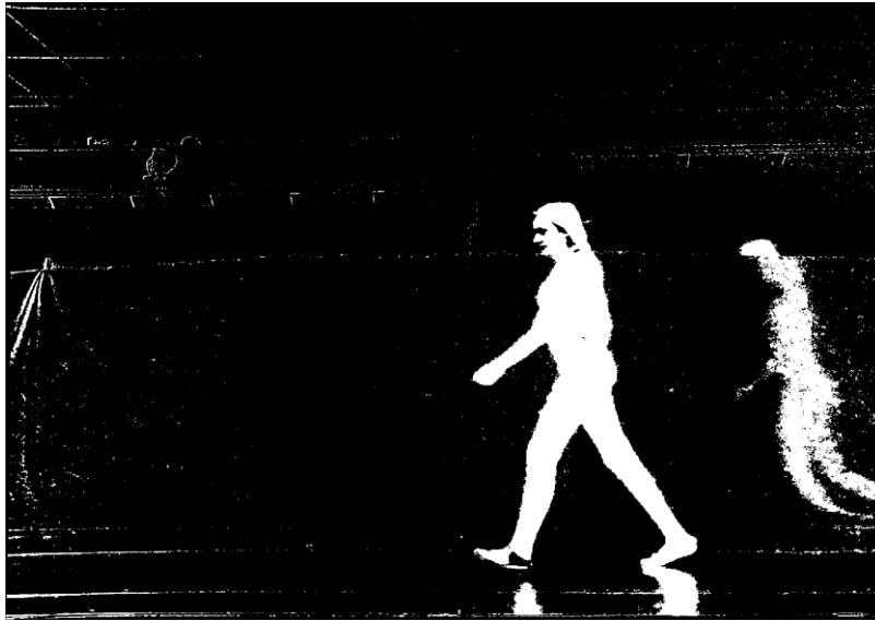
Figure 13. The final segmentation {}^I M_{sub} obtained by applying the threshold Th .
