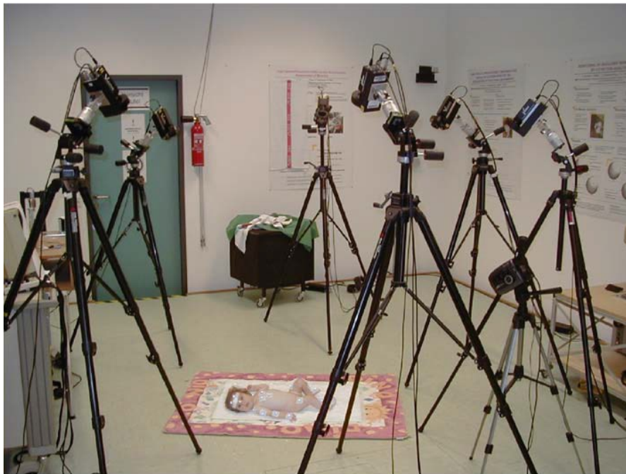
Figure 60. Marker-based system for the general movement analysis of newborns at risk for developing spasticity.
