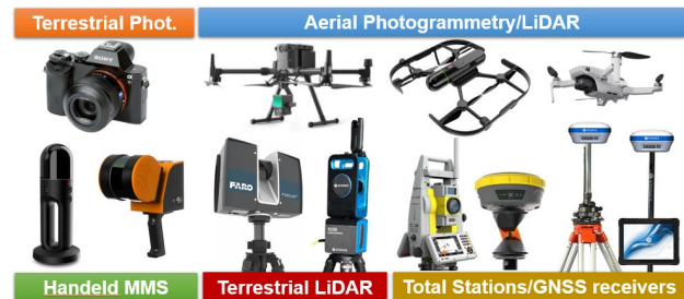
Figure 3. Instruments used in the survey of terrestrial case
