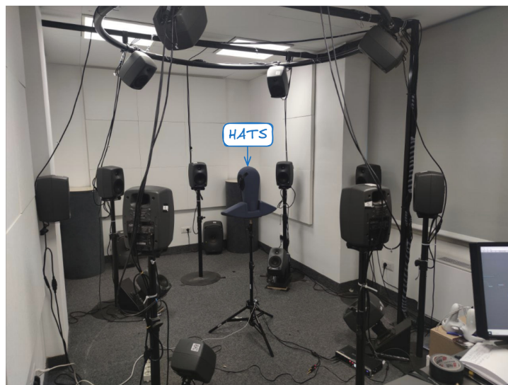
Figure 5. BRIR measurements within the ASL, with the HATS wearing the HAs placed at the 0 cm off-center position from the sweet spot.
