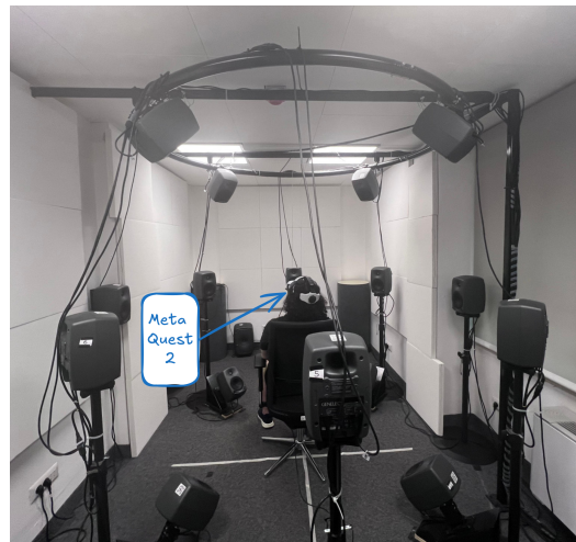
Figure 4. Picture of the VR system inside the ASL during the execution of a speech intelligibility test on a listener.
