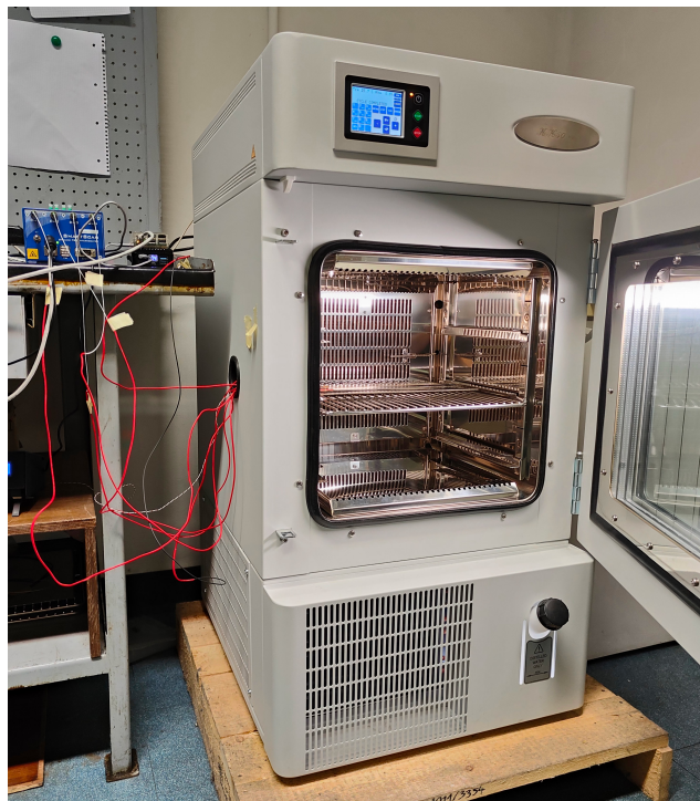
FIGURE 2.22: PhotoNext FBG Data Analyzer Laboratory Tests - The configuration employed for the temperature measurement test, featuring the climatic chamber housing the network of sensors. This image was taken from [51].
