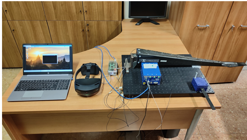
FIGURE 2.25: PhotoNext FBG AR Viewer Laboratory Tests - A picture of the settings used for strain measurement tests, featuring the CFRP, the instrumented tail of Anubi, and the Microsoft HoloLens. This image was taken from [54].
