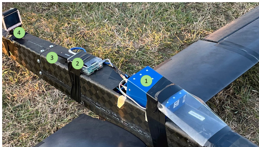
FIGURE 2.30: Middleware, Cloud Database, and 3D Viewer Flight Tests - A close-up of the instrumentation installed above Anubi during the three flight test groups conducted at the Tetti Neirotti airfield: SmartScan interrogator (1), Raspberry Pi (2), Internet Key (3), action cam (4). The action cam was utilized to capture graphic documentation of the flights. This image was taken from [35].
