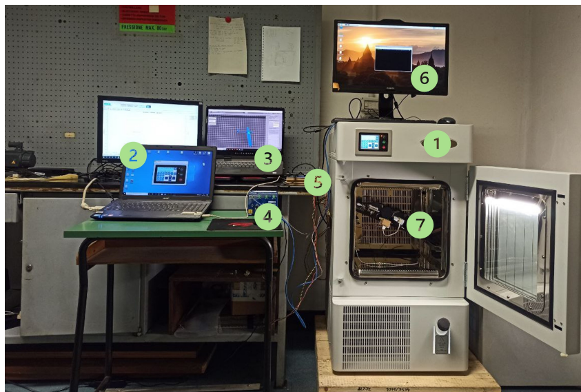
FIGURE 2.17: Middleware, Cloud Database, and 3D Viewer Flight Tests - Setup utilized for the strain measurement test, including: the climatic chamber (1), monitored by two screens (2), a laptop running the 3D Viewer application (3), the interrogator (4), the Raspberry Pi (5), with its operations monitored on screen (6), the test sample equipped with the FBG sensor (7). This image was taken from [35].
