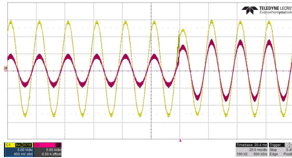
Fig. 6.8 An output voltage response of a cascaded dual loop controller on oscilloscope.
