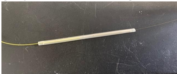
b) Fusion area protected by plastic cover
