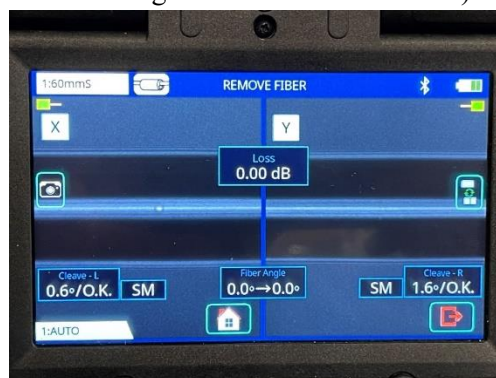
e) Splice fiber with a loss of zero
