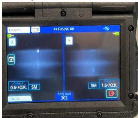
c) A moment before the fusing starts d) Fusing phase
