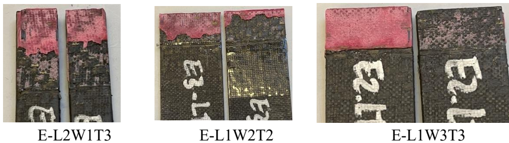
Figure 6.8. Failure surfaces of the specimens after the test
