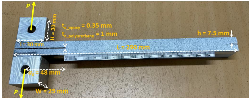
Figure 3.4 DCB specimen geometry: t_a =adhesive thickness, a_0 =initial crack length from the loading line, W = width of the specimen, L =length of the specimen, h =substrate thickness, H =block height, l =block width.
