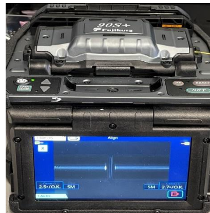
a) Placing the cleaved fibers in the slicer b) Bringing the fibers near each other
