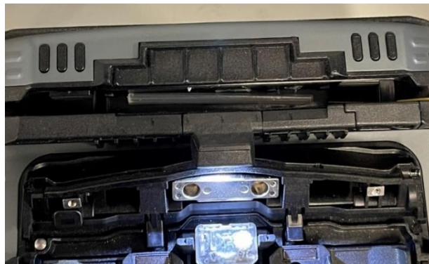
a) Exposing the fiber fusion area with the plastic cover to heat
