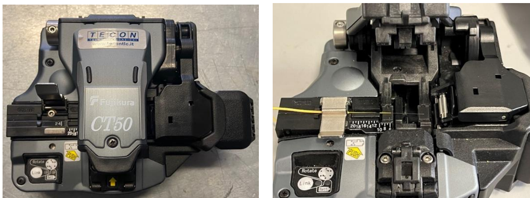
a) Cleaver with closed lid b) Cleaver with fiber placed inside
