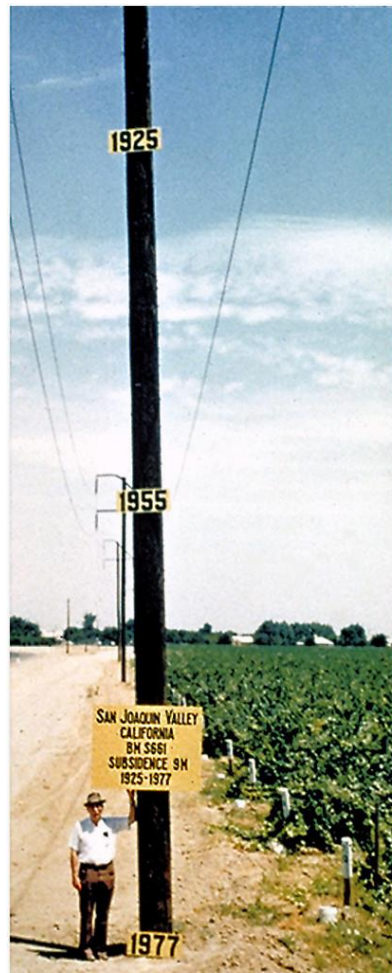
Figure 2.1: The San Joaquin Valley (California) subsidence case. Photo shows location of maximum subsidence of approximately 9 m from 1925 to 1977 caused by groundwater pumping. Photograph by R.L. Ireland featuring Dr. J.F. Poland (1977).
