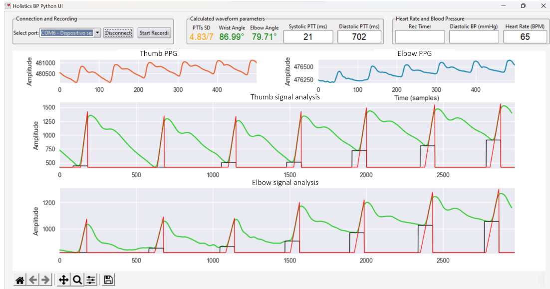
Figure 6.4: Graphic User Interface used by the device in the BP assessment. The upper plots show the thumb signal (red) and elbow signal (blue). Bottom plots depict the intersecting tangent being extracted from gathered signals for PTT estimation.
