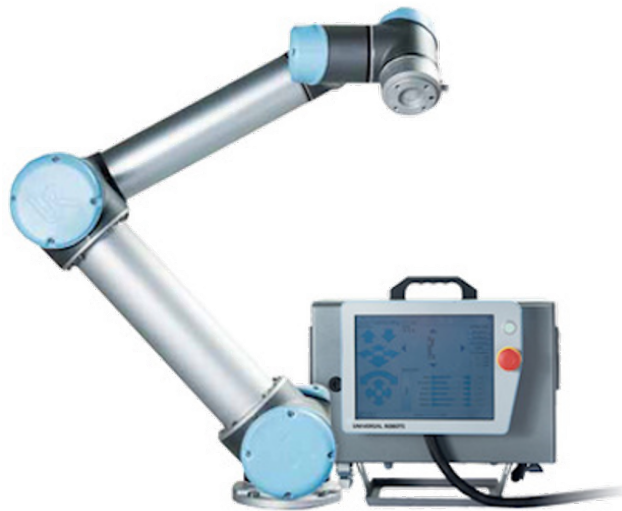
Fig. 4.5 UR5 CB3-series with its control unit and its teach pendant.
