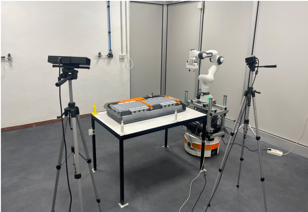
Fig. 5.37 Final setup with the solid markers used to define the Kinect reference frame.
