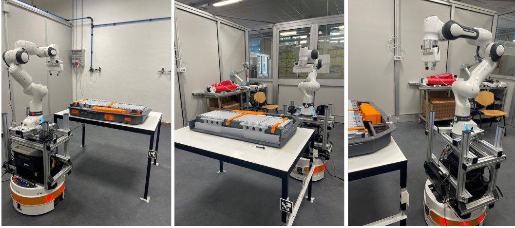
Fig. 5.11 Setup of the worktable, with the Aruco markers, and the robotic system with the Realsense.
