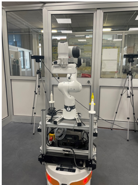
Fig. 5.23 Setup for the identification of the transformation matrix Kinect-Map.
