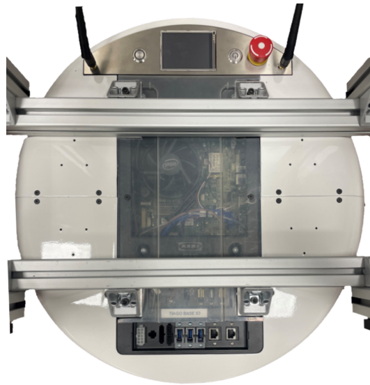
Fig. 5.6 TIAGo Base and aluminum structure fixed on it.
