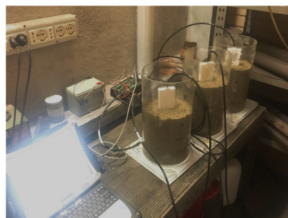
Figure 1. Experimental setup of the three mesocosms with the sensors for monitoring electrical conductivity and permittivity and the connection with the datalogger and the laptop.
