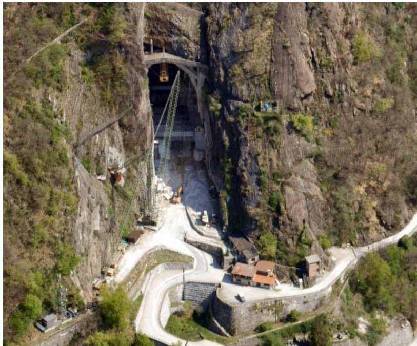
Figure 1. Aerial front view of the adit, access ramp and upper yard of the Cava Madre of Candoglia, from where the marble is extracted for the continuous renovation of the external casing of the Milan Cathedral.
