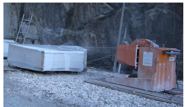
Figure 5. Left: operation scheme of the diamond wire system. Right: example of use of diamond wire system for secondary cuts at the front yard of Cava Madre, before transportation to the local workshop in Candoglia
