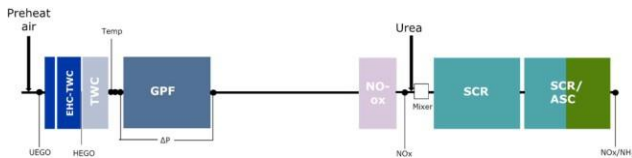
Figure 7: Final Exhaust Aftertreatment Configuration.
