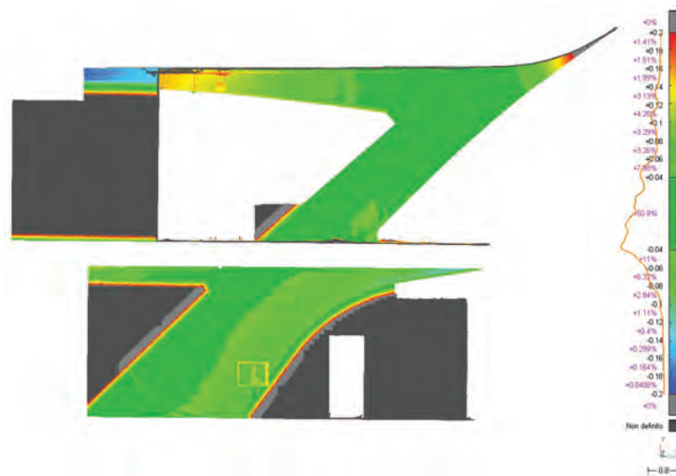
8a 2.2: Discrepancy analyses conducted between the reality-based model (created from LiDAR data) and the 3D model from Pier Luigi Nervi's drawings after the co-registration procedure.
