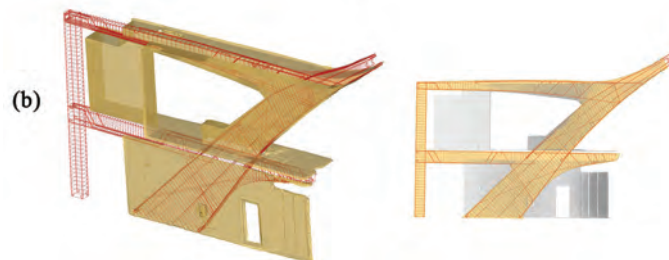
8a 2.4: (a) Integration of the extrados of the P12 pillar module in the reality-based point cloud. (b) 3D models of the internal structural elements developed from the design phase.
