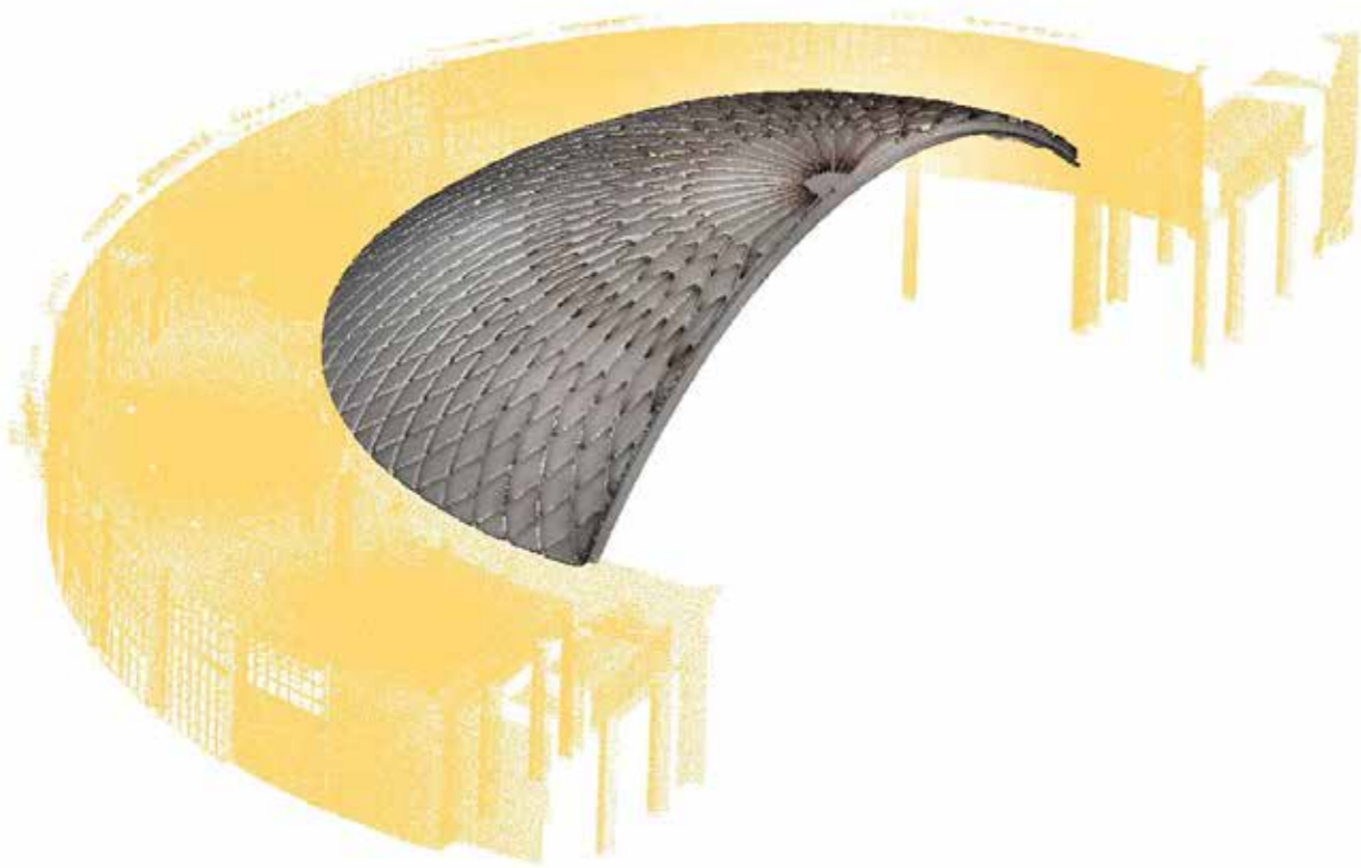
3b 2.3: LiDAR cloud of the apse of Hall B, highlighting the spherical dome studied. [Point cloud of the apse is segmented by the other components of the 3D model.]
