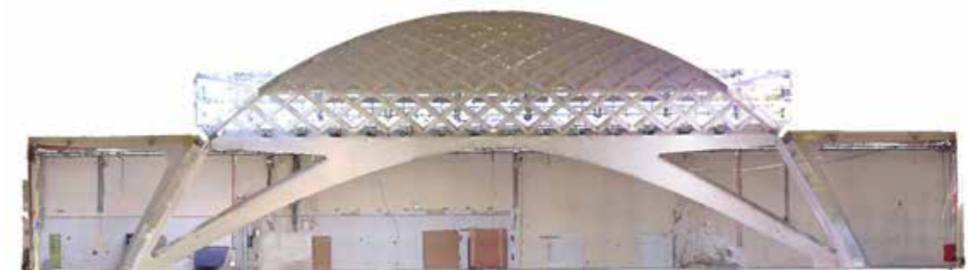
3a 6.5: A projected section of the LiDAR point cloud of Hall C.
