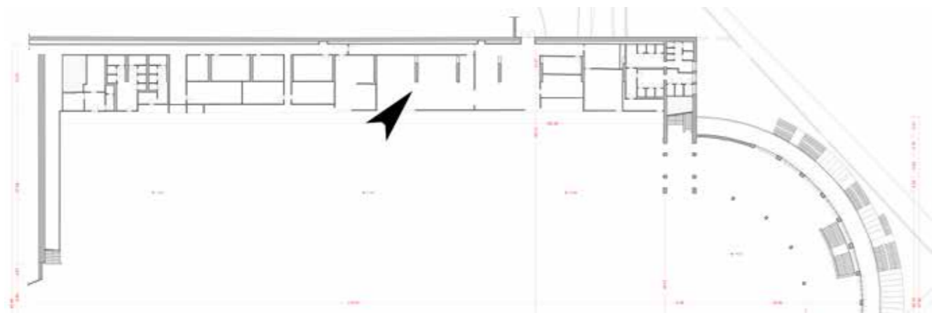
3a 7.3: The combination of clouds from consecutive trajectories in the north rooms of the ground floor of Hall B and the corresponding architectural drawing to a scale of 1: 200. It was thus possible to recognize and measure the complete spatial configuration of the large, inclined pillars incorporated into the rooms.
