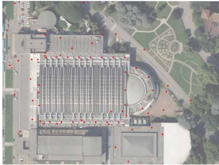
3a 5.3: Distribution of control points for UAV photogrammetric survey
