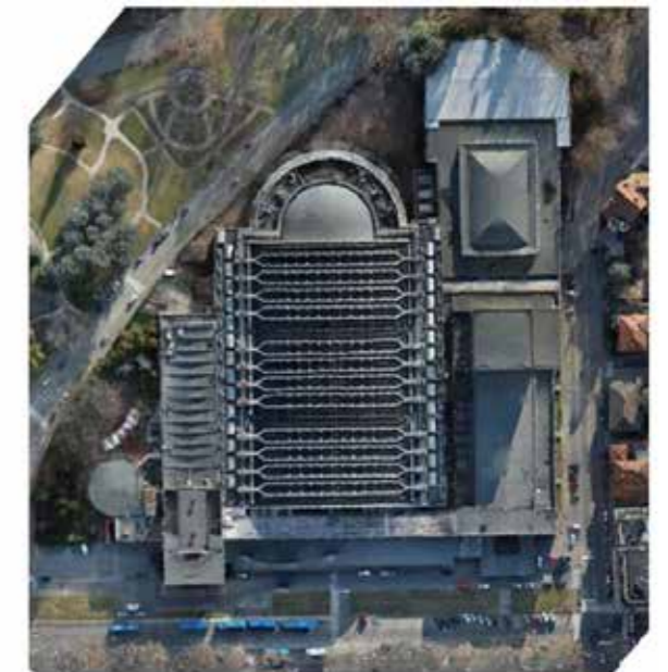
3a 5.6: Metric products achieved using the photogrammetric technique. Left, DSM. Right, orthomosaic.
