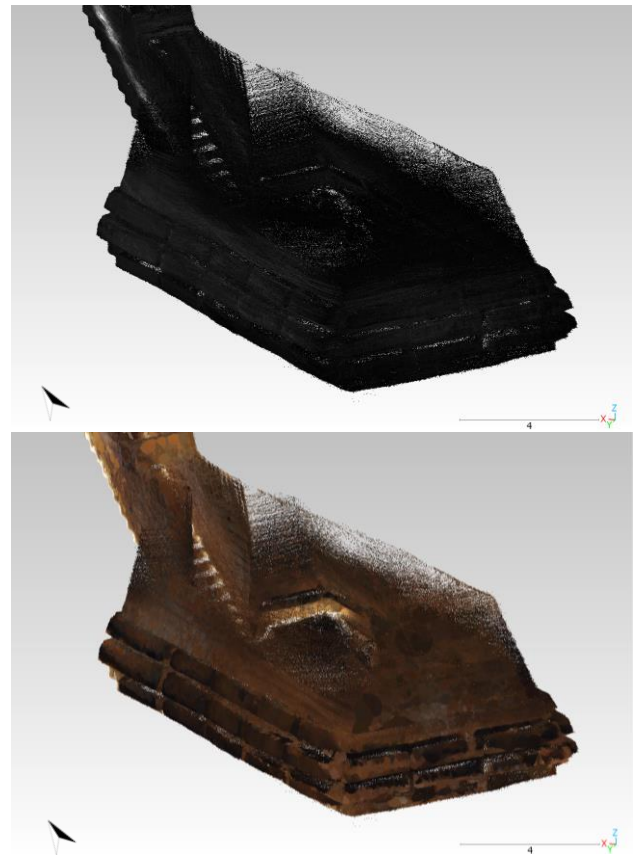
Figure 11. In the upper part, the MMS point cloud shows the intensity scalar field, the LiDAR intensity function recorded as the laser beam's return strength. At the bottom, the same point cloud is colored using the radiometric information extracted from the SP model.
