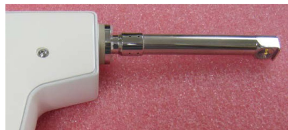
Fig. 1 Prototype of manual probe for intraoral use
