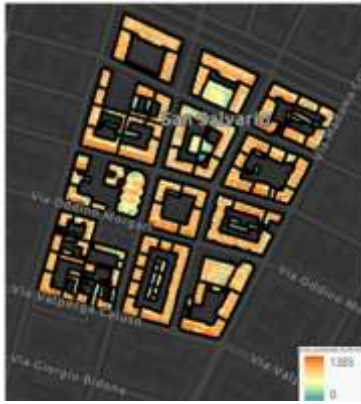
Figure 5: Solar Potential Estimation for all the buildings in the selected locality of San Salvario
