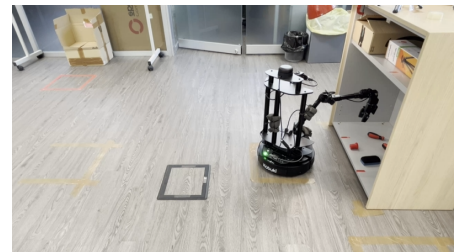
(c) Arm moves to reach the pre-grasp pose.
