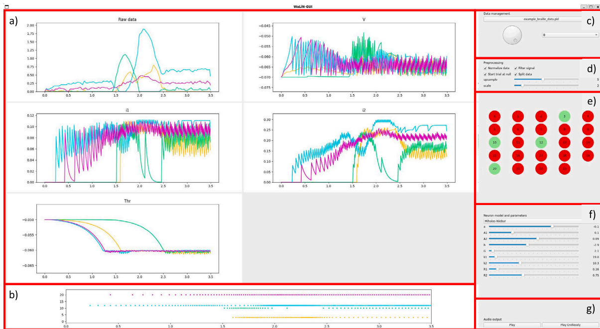
Fig. 1. The Win-GUI: on the left-hand side are the plots used to visualize the input data and analyze the neuron dynamics (a, b), on the right-hand side are the data (c, d), channel (e), parameter (f), and audio (g) settings.
