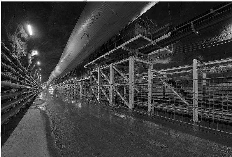
Figure 6.6 Horizontal belt storage. (Courtesy of Marti Technik.)
