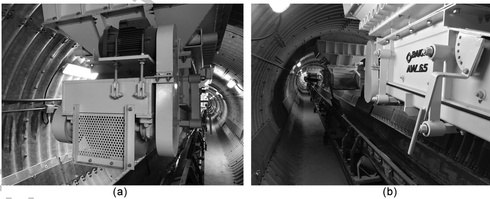
Figure 6.23 Automatic load system for aggregates (a and b). Emergency loading system for aggregates (c).
