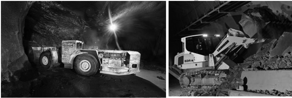
Figure 6.13 GHH diesel (can be also electric-driven) LHDs are particularly compact with a good operator's position (a) and a crawler Liebherr L634 (b).
