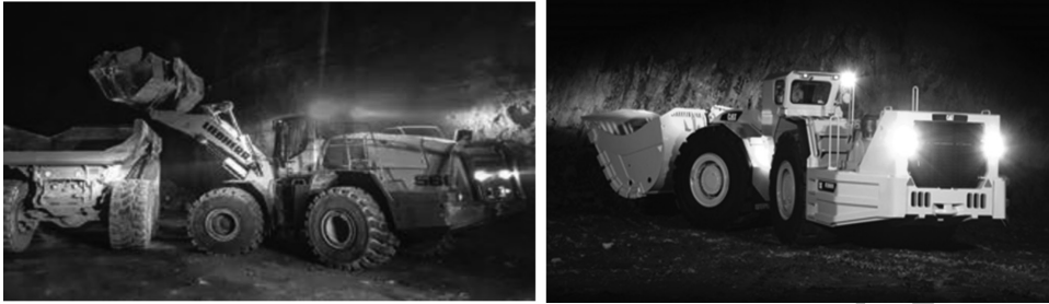
Figure 6.12 Example of wheel loader and LHD. The L566 is loading dump trucks with a capacity of up to 45 ton (a) and the largest loader in Cat's LHD line-up, the R3000H (b). (Courtesy of Bringiotti.)
