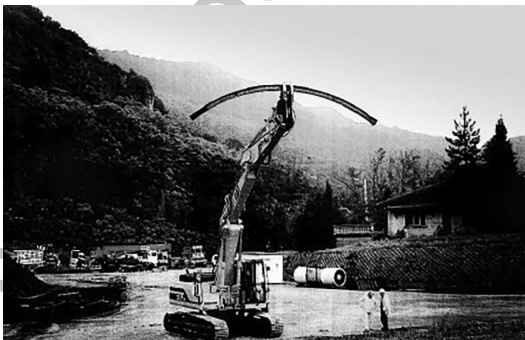
Figure 6.10 Clamp for setting steel ribs.
