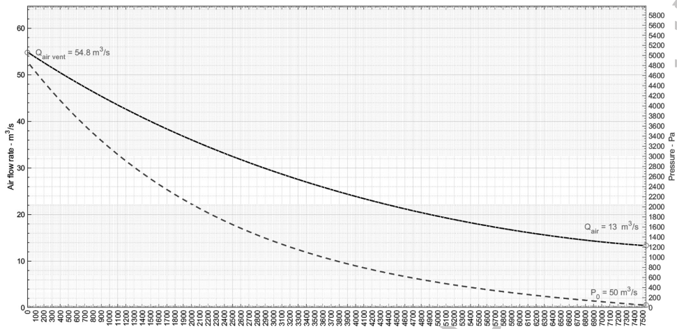
Figure 6.50 Pressure and velocity (flow rate values Q_0 vs Q_1 ) trends along tunnel ducts.
