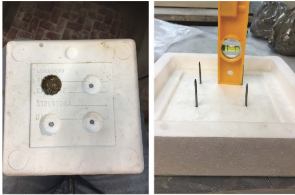
Figure 3. Polystyrene support used for the samples production.
