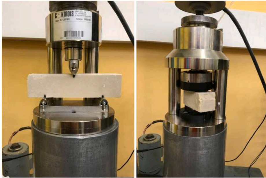
Fig. 6. Left: tensile strength assessment performed according to the 3-point flexural test. The frame for the three-point flexural test is depicted. Right: uniaxial compression strength assessment, performed by using the compriator. Both depicted devices are in compliance with the CEN (2016).
